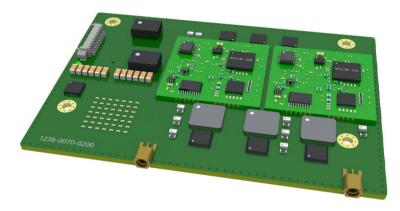
3D model of the new receiver prototype with IDM integrated
