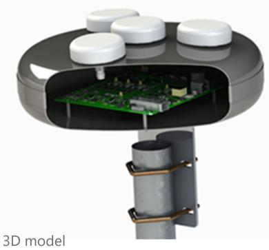
3D model of the CRPA prototype
